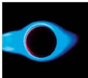
High flame temperature based on cyclone swirl
