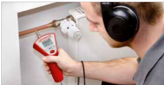
Acoustic leak detection of heating installations
